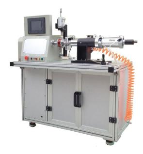
•Name: Motor Stator Coil Winding Machine Character: Arrange 30 floors can precision, not fold line. Automatic tracking, automatic correction.. With the function of first in line.
