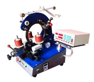
•Name: Toroidal winding machine
