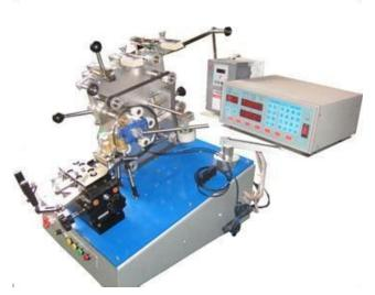
•Name: Toroidal winding machine
