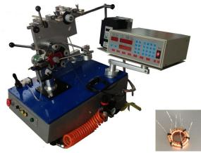
•Name: Toroidal winding machine This machine is to order products.
