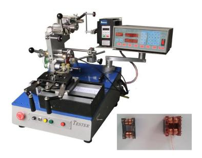
•Name: UT series of coil winding machine
