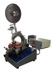
•Name: Toroidal coil taping machine
