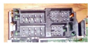
The 2 big ISO connectors on the left are for 12V, speakers, etc. On the right, bottom position is the Blue connector for the CDC and above that, on the right hand side the Yellow connector is present that is connected to your display/steering wheel controls. Left next to the Yellow connector the Green fits in and that is the connector that you need to connect the AUX input.
